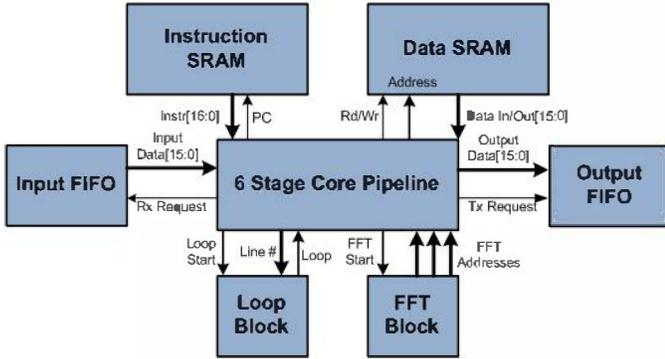
Fig. 3. Single core block diagram consisting of the 6 stage pipeline, instruction and data memory, and input/output FIFO's.
