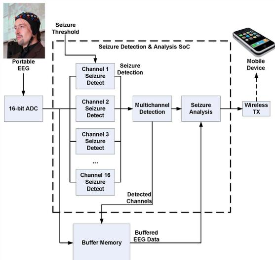
Fig. 1. Proposed multi-channel seizure detection and analysis architecture. 16 single channel detection circuits are instantiated and passed to a threshold detector to confirm a seizure. Subsequently, analysis circuitry is enabled, which perform frequency and energy recording of seizure in certain frequency bands.
