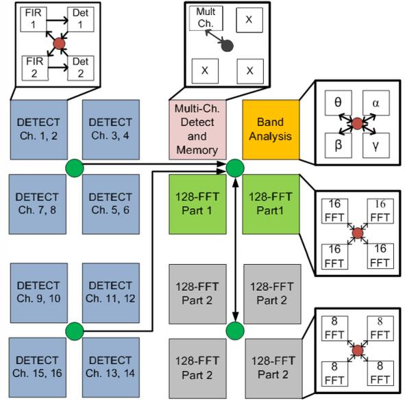
Fig. 4. Mapping of the seizure detection and analysis hardware block onto the many core platform. The implementation supports 16 EEG channels mapped onto 61 cores.
