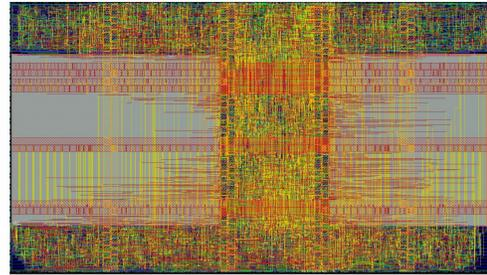
Fig. 5. Layout of a single processor core. The blocks on the left and right side are the instruction and data SRAM memories, respectively.
